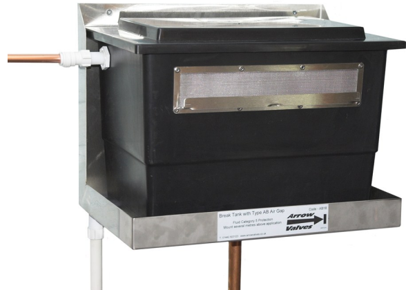
AB18 – Cistern with Type AB air gap. Supplied complete with stainless steel screened slot, wall bracket incorporating drip tray. Also supplied - float valve with pipe connection and servicing valve
