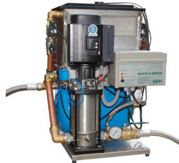
Model 5-8 Variable speed Stainless tank, twin inlet solenoid. Height 775 mm. High flow 2 Lt/s output
