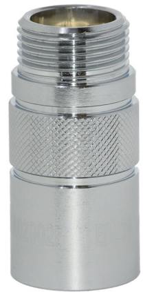
ED15FM235 Double Check Valve designed specifically for bath shower hoses – with optional Automatic Flow Limiting cartridge. Female Inlet, EPDM washer supplied
