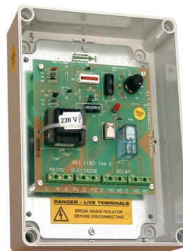
Level Controller (lid removed) acts as junction box – IP65 Single unit dims -
