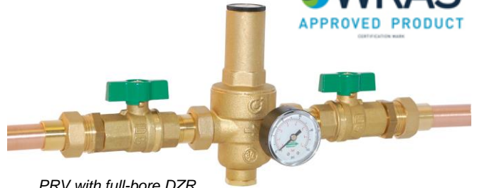
PRV with full-bore DZR servicing valves and solder unions for secure fitting to copper pipe.
