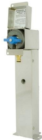
Model SPTG Low level Standpipe with Double Check Valve for Fluid Category 3 protection. Flange enables mounting to flat surface – concrete or flat roof for window cleaning and roof garden watering
